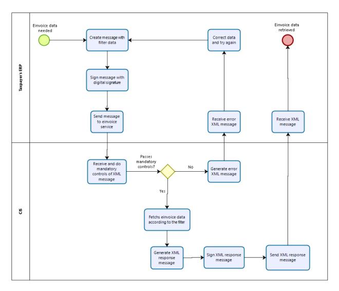
If needed, Taxpayer's ERP can use einvoice service method to retrieve einvoice data from CIS. To successfully retrieve data, ERP must issue signed message with filter data.
